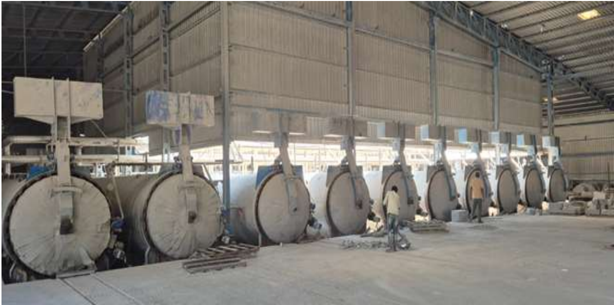
Figure 6 Steam Curing Process (Autoclave Reactor)
